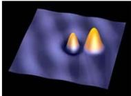
Scientists at IBM's Zurich Research Labb manipulate and control the charge state of individual atoms. This ability to add or remove an electron charge to or from an individual atom can help expand the scope of atom-scale research. Switching between different charge states of an individual atom could enable unprecedented control in the study of chemical reactivity, optical properties, or magnetic moment.
