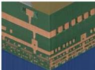
IBM demonstrates the first-ever manufacturing application of "self assembly" used to create a vacuum—the ultimate insulator—around nanowires for next-generation microprocessors for its "airgap" chip technique.
