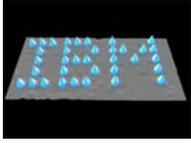
IBM Fellow Don Eigler is the first to controllably manipulate individual atoms on a surface, using the STM to spell out "I-B-M" by positioning 35 xenon atoms, and in the process, perhaps creating the world's smallest corporate logo.
