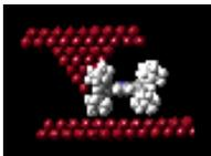
IBM Zurich scientists extend STM manipulation techniques to position individual molecules at room temperature for the first time.
