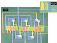
IBM researchers build the first complete electronic integrated circuit around a single "carbon nanotube" molecule, a new material that shows promise for providing enhanced performance over today's standard silicon semiconductors. Importantly, the breakthrough builds on standard semiconductor processes, using a single molecule as the base for all components in the circuit.
