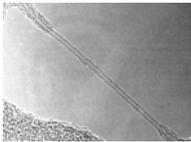
Scientists at IBM and NEC independently discover single-wall carbon nanotubes and the methods to produce those using metal catalysts.
