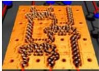
IBM researchers build world's smallest operating computing circuits using a molecule cascade, wherein molecules move in a manner analogous to falling dominos.
