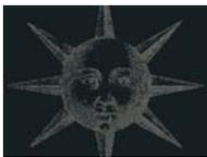
IBM Zurich researchers in collaboration with scientists from the ETH Zurich demonstrate a new, efficient and precise technique to print at the nanoscale, using particles only 60nm in size. The method could advance the development of nanoscale biosensors, of lenses that can bend light inside future optical chips, and the fabrication of nanowires that might be the basis of tomorrow's computer chips.
