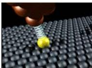
IBM scientists measure the magnetic anisotropy of a single atom. This property determines an atom's ability to store information. The breakthrough is a major step in understanding the ability for single atoms to maintain a specific magnetic direction, making them suitable for future data storage applications.
